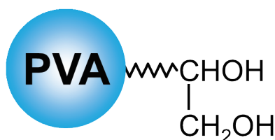
Fig. 1. Schematic diagram of VN-50 packing material
